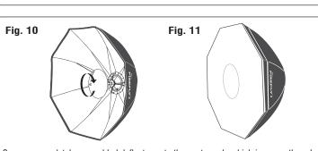
Screw a completely assembled deflector onto the center pole which is screw thread. Use without covering a front diffuser to enjoy beauty dish lighting. See fig. 10 Cover the front of Firefly Beauty Box with the included diffuser for softer light See fig. 11
