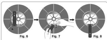
Rotate the attached arm on the swivel bracket anticlockwise while pressing the button attached to the ring. Locate the hole in the arm over the stud then release the button so that the stud protrudes through the hole in the arm which will lock it securely into place. See fig. 6, fig. 7 and fig. 8
