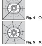
The grooves inside of the runners should connect with two projecting parts in the center pole. When the runners and center pole grooves are connected, all the stretchers should be straight and be equal. See fig. 3, fig. 4 and fig. 5
